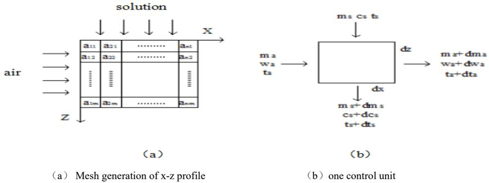
Fig.3. discrete grid diagram of the cross-flow dehumidifier
