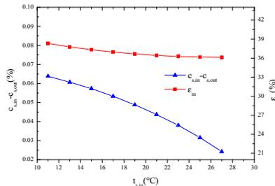
Fig.13 Influence of  $t_{s,in}$  on  $c_{s,in}-c_{s,out}$  and  $\epsilon_m$
